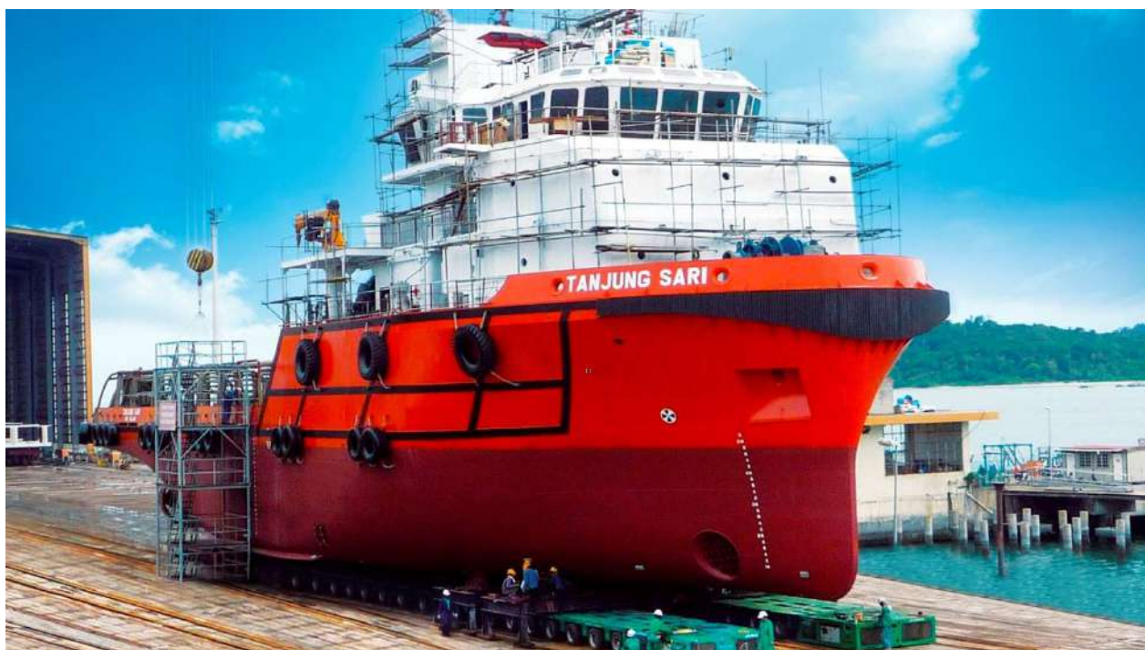
Making a double 90-degree turn maneuver and travelling a distance of 250 metres to the boat-lift-system, the Tanjung Sari Tugboat weighing 1500 tonnes was shifted utilizing 56 axle lines Goldhofer Self-Propelled Modular Hydraulic Controlled Transporter on the 12th July 2009 at Boustead Naval, Lumut Shipyard.
