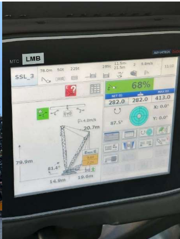
Transportation of 184T Module from Samalaju Port to OCI ME1 Samalaju Plant utilising SCHEUERLE SPMT 30 x 2 (60) axeline and 2 PPU. Using 800T DEMAG CC3800-1 with Boom Booster lifting Module + Accessories with a total load of 282T on top of another Module for the final installation.
