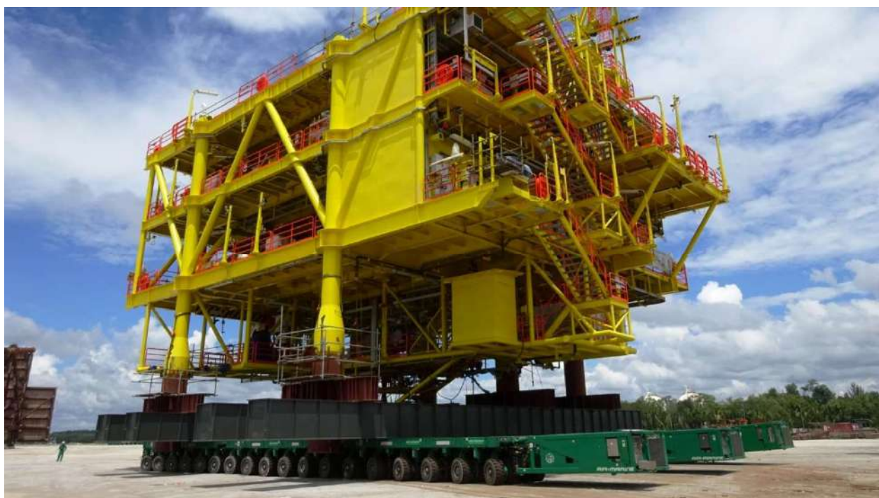
Shifting of 812Te BP-A (Bunga Pakma – A) Topside by utilising our 54 axelines of Scheuerle 4th Gen. Self Propelled Modular Trailers (SPMT's) coupled with 3units hydraulic Powerpack units from the fabrication area to the quayside for our prestigious and distinguished clients Oceanmight Sdn Bhd on the 11th of August 2017, at their fabrication yard in Kuching, Sarawak, for Repsol Oil & Gas Malaysia Ltd. The synchronised shifting operation lasted for around one hour and subsequently upon reaching the quay side, the Topside was loaded out to the already pre-ballasted 330' flat top ballastable barge by utilising 20nos of our diesel driven ballast pumps.
