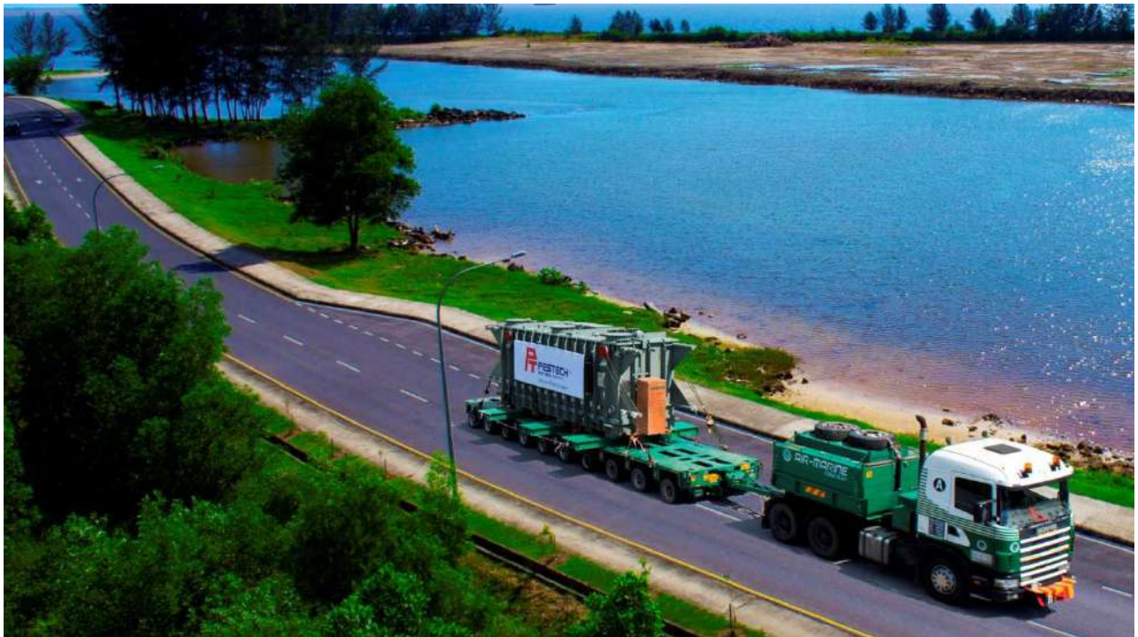
✓ Overland transportation of four (4) units of 275/35KV 180 MVA Power Transformers for our esteemed client, Pestech Sdn Bhd, from Bintulu Port to Samalaju project site, Bintulu. The cargo weighing 150 tonnes each, measuring 3.39m(H) X 2.80m(W) X 10.43m(L) was transported utilizing our hydraulic multi-axle modular trailer towed by high-powered heavy duty primemover.
