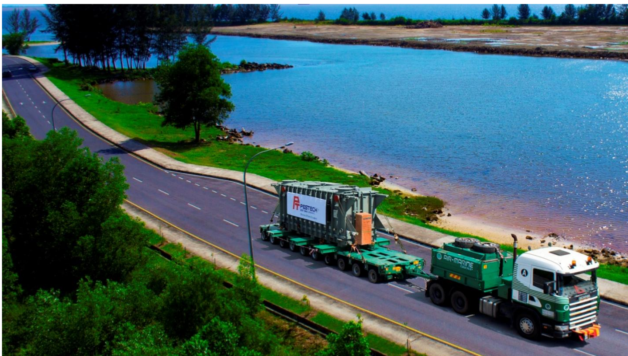
✓ Overland transportation of four (4) units of 275/35KV 180 MVA Power Transformers for our esteemed client, Pestech Sdn Bhd, from Bintulu Port to Samalaju project site, Bintulu. The cargo weighing 150 tonnes each, measuring 3.39m(H) X 2.80m(W) X 10.43m(L) was transported utilizing our hydraulic multi-axle modular trailer towed by high-powered heavy duty primemover.
