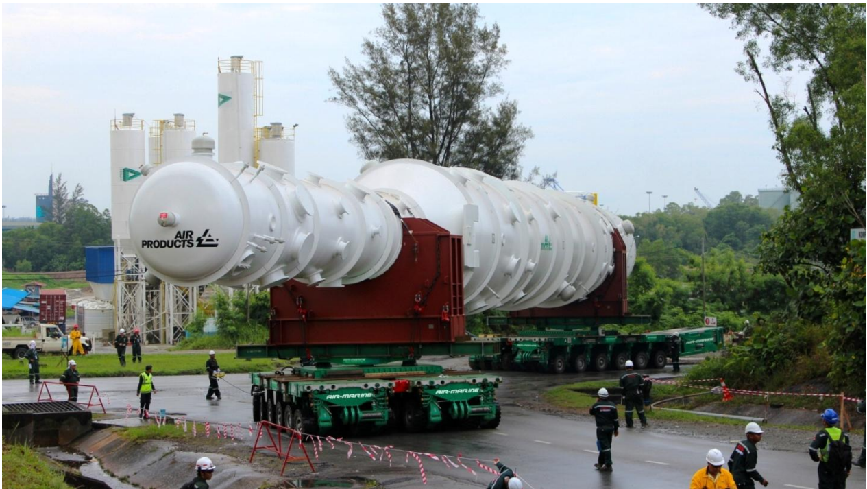
On 11th May 2014, AIR-MARINE transported a 300Te - 56m long, 5.4m wide and 6.1m high - Main Cryogenic Heat Exchanger (MCHE) from the port of Bintulu, Sarawak, Malaysia to the Petronas LNG Train 9 (project site). For this transportation, AIR-MARINE utilized its trusted Scheuerle 4th Gen SPMT's; which were assembled in 6 axleline in 4-file (side by side/double) in Dolly configuration, c/w 300Te Bolsters (Turntables) and a 350kW Diesel Driven Powerpacks on each 4-file system. In total there were 24 axlelines SPMT's + 2PPU's + 300Te Bolsters which were utilised for the entire transport operation.
