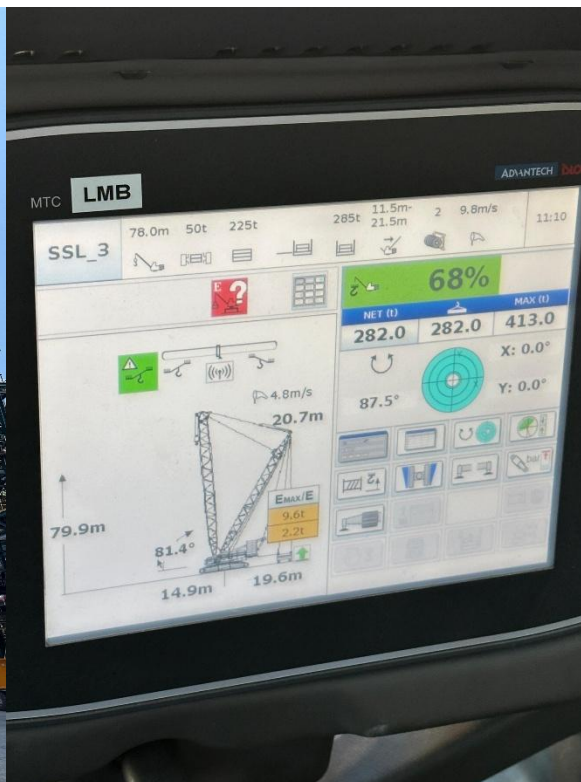
Transportation of 184T Module from Samalaju Port to OCI ME1 Samalaju Plant utilising SCHEUERLE SPMT 30 x 2 (60) axleline and 2 PPU. Using 800T DEMAG CC3800-1 with Boom Booster lifting Module + Accessories with a total load of 282T on top of another Module for the final installation.
