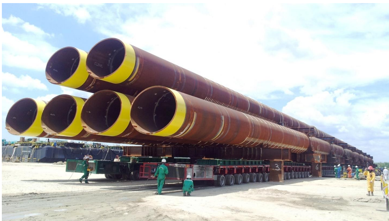
✓ AIR-MARINE was contracted to load-out piles for KHL and KPOC from the fabricator's yard onto a barge. The 146 meter length and 3,582 tons weight of the pile set a record for the second longest and heaviest load-out in the world. We did this remarkable job using our 156 axle-lines of multi-axle trailers and 8 PPU. The combined transport weight was above 4300te. AIR-MARINE did load-out of 2 set of piles for this project.
