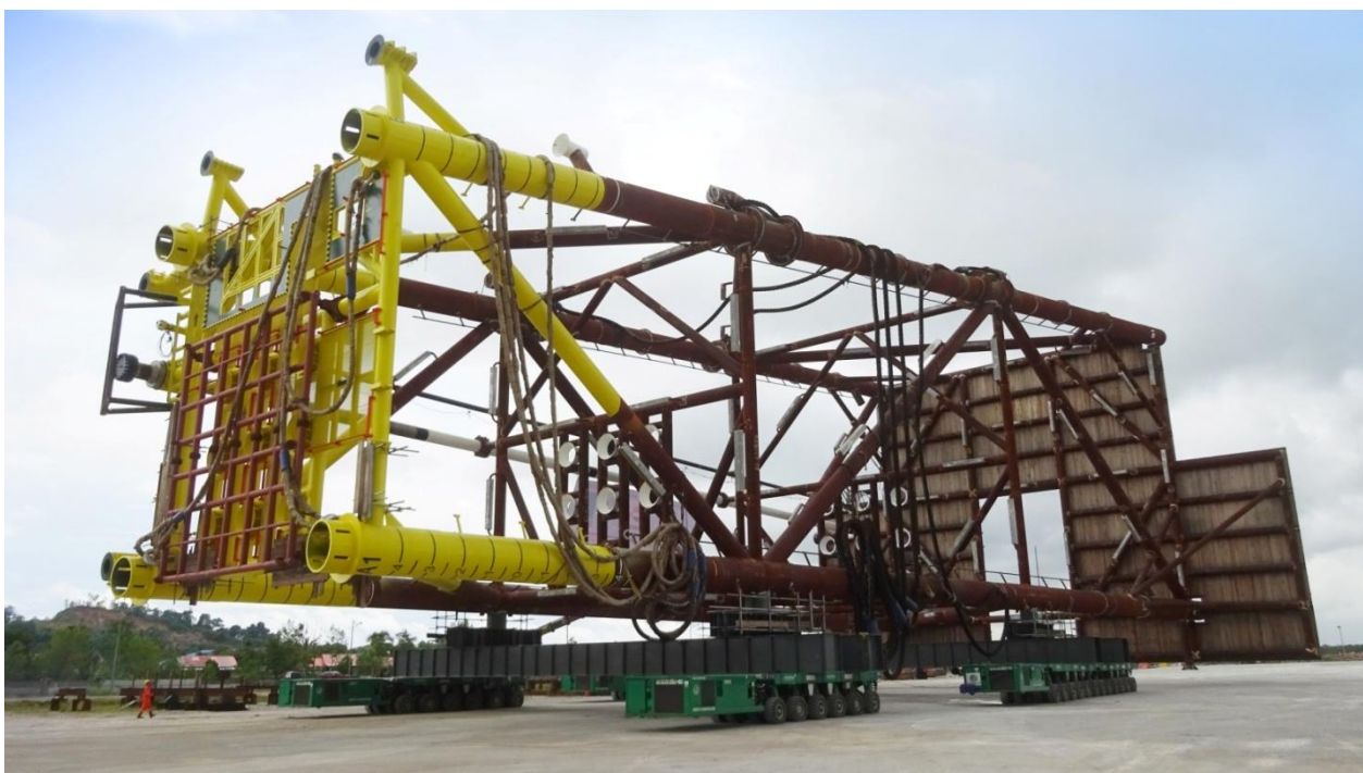
Shifting of 766Te BP-A (Bunga Pakma – A) Jacket by utilising our 36 axelines of Scheuerle 4th Gen. Self Propelled Modular Trailers (SPMT's) coupled with 4units hydraulic Powerpack units from the fabrication area to the quayside for our prestigious and distinguished clients Oceanright Sdn Bhd on the 16th of August 2017, at their fabrication yard in Kuching, Sarawak, for Repsol Oil & Gas Malaysia Ltd. The synchronised shifting operation lasted for around one hour and subsequently upon reaching the quay side, the Jacket was loaded out to the already pre-ballasted 330' flat top ballastable barge by utilising 20nos of our diesel driven ballast pumps.
