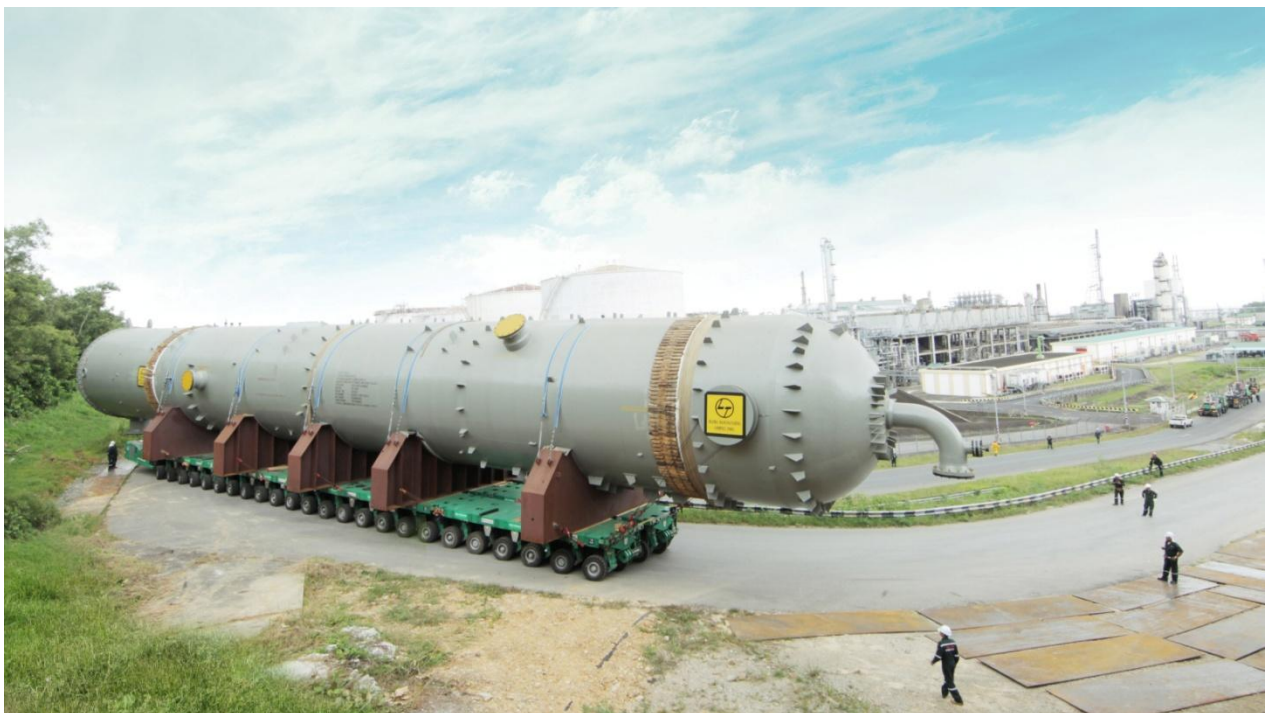
The successful accomplishment of heavy lift transportation for one (1) unit of Deep AGR Absorber Column for Petronas-MLNG with a combined weight of 1480 metric ton hauled from Bintulu Port to Petronas MLNG – Train 9 project site using 48 axle line SCHEUERLE Self Propelled Modular Transporter (SPMT). The sophisticated state-of-the-art equipment, excellent teamwork, cooperation and expert transport engineering have contributed to the success of this move on public road unmatched by any others in Malaysia.
