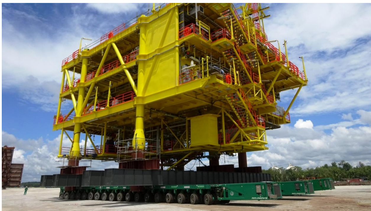
Shifting of 812Te BP-A (Bunga Pakma – A) Topsides by utilising our 54 axles of Scheuerle 4th Gen. Self Propelled Modular Trailers (SPMT's) coupled with 3 units hydraulic Powerpack units from the fabrication area to the quayside for our prestigious and distinguished clients Oceanright Sdn Bhd on the 11th of August 2017, at their fabrication yard in Kuching, Sarawak, for Repsol Oil & Gas Malaysia Ltd. The synchronised shifting operation lasted for around one hour and subsequently upon reaching the quay side, the Topsides were loaded out to the already pre-ballasted 330' flat top ballastable barge by utilising 20nos of our diesel driven ballast pumps.
